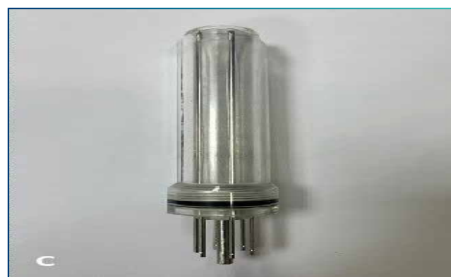
Figure 3: (A) Planned treatment isodose lines (75% – dark blue, 100% – yellow, 200% – red) covering the clinical target volume (dotted blue line) and sparing of the rectum (dotted yellow) and bladder (dotted red); (B and C) In-house developed six-channel intravaginal brachytherapy cylinder (B) Individual components; (C) Assembled cylinder.
