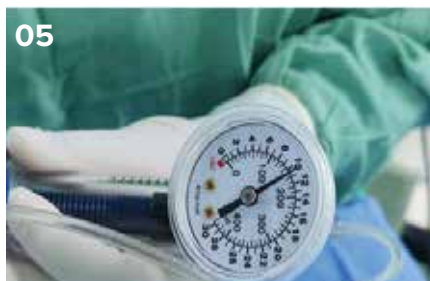
Figure 5: Pressure of about 10 Bars was maintained for 2 minutes.
