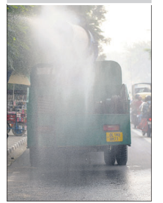
An anti-dust gun sprays water droplets to curb air pollution. ANI
